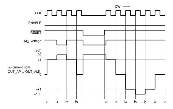
Setting the RESET signal Low causes the outputs to be put in the Initial state and the Mo output to be driven Low (Initial state: A-channel output current is at its peak (100%)).
