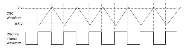
Figure 2 Timing Waveforms (OSC Signal)
