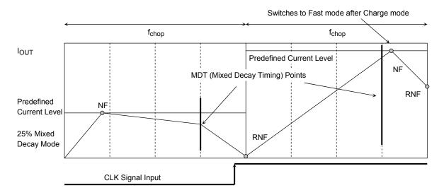
• When the output current value > predefined current level in Mixed Decay mode
