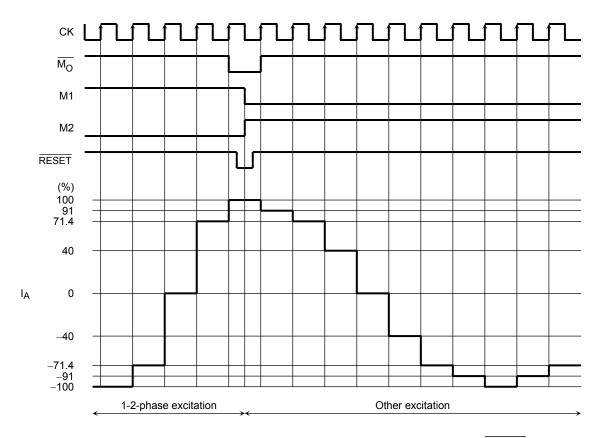
It is recommended that the state of the M1 and M2 pins be changed after setting the  $\overline{RESET}$  signal Low during the Initial state (MO = Low). Even when the MO signal is Low, changing the M1 and M2 signals without setting the  $\overline{RESET}$  signal Low may cause a discontinuity in the current waveform.
