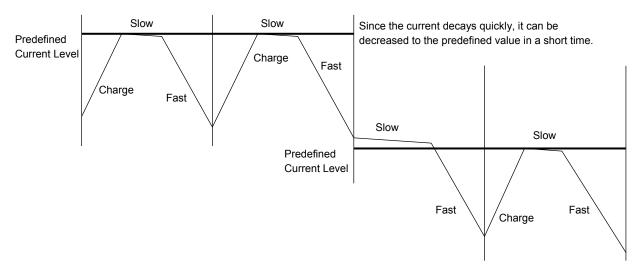
• Decreasing the current with a low decay rate (The current decay rate in Mixed Decay mode is the ratio between the time in Fast-Decay mode (discharge time after MDT) and the remainder of the period.)
