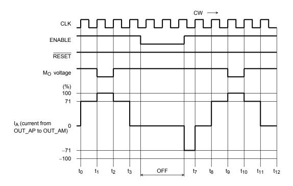
Setting the ENABLE signal Low disables only the output signals, while internal circuitry other than the output block continues to operate in accordance with the CLK input. Therefore, when the ENABLE signal goes High again, the output current generation is restarted as if phases proceeded with the CLK signal.
