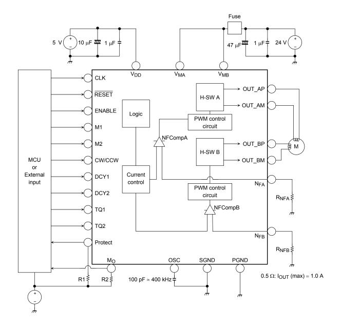
Note: Capacitors for the power supply lines should be connected as close to the IC as possible.
