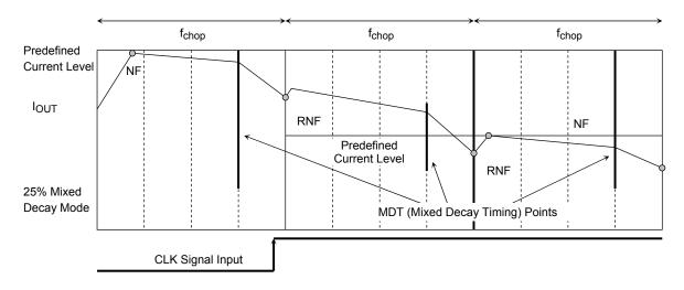
\*: Even if the output current rises above the predefined current at the RNF point, the current control mode is briefly switched to Charge mode for current sensing.
