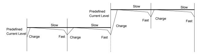
• Decreasing the current with a high decay rate (The current decay rate in Mixed Decay mode is the ratio between the time in Fast-Decay mode (discharge time after MDT) and the remainder of the period.)
