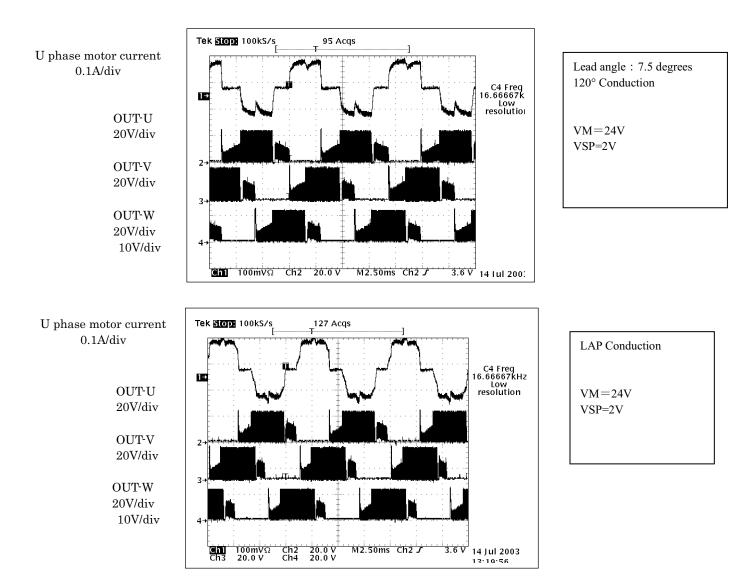
Using the motor at higher than withstand voltage of comparator.
